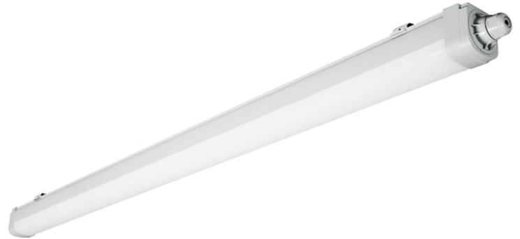
START Waterproof Slim is a LED integrated polycarbonate housing luminaire with easy to access electrical terminal through bayonet lock end caps and tool-free electrical connection due to push-in terminal. Flexible installation as mounting brackets can be positioned freely on the luminaire. 7300 / 3800lm (selected by DIP switch), 52.5 / 26W, 139 / 146lm/W and 100,000 hours lifespan L70B50. SDCM < 5; IP66; IK08; Class II; 1540mm x 70mm x 73mm.
